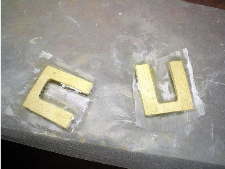
Retract mount covers, made from 12mm balsa, glassed with 3/4oz and screwed to bearers. Removable for retract maintenance
