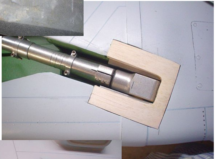
Retract mount covers, made from 12mm balsa, glassed with 3/4oz and screwed to bearers. Removable for retract maintenance
