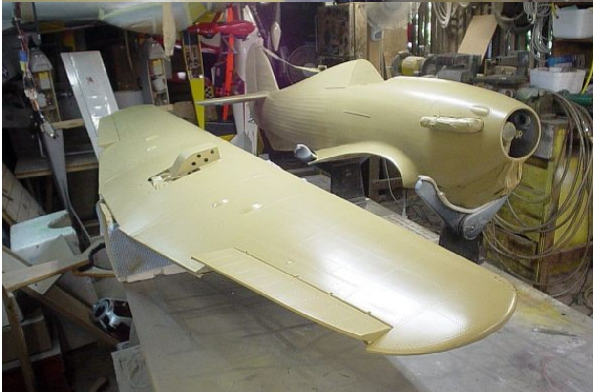
Another 10 bucks worth of masking (number 3) and a coat of Mid Stone completed. Dark Earth to go....
